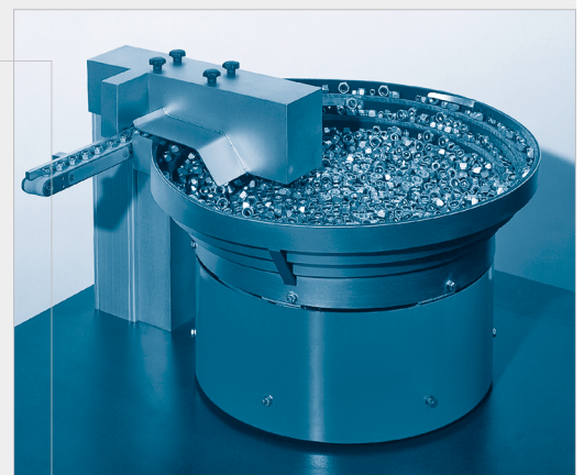
sortimat SMIK – the integrated vision system for bowl, step, and drum feeders
